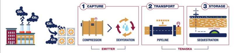
Curious about how carbon capture and storage (CCS) works? Our CCS 101 guide breaks down the fundamentals, from how CO<sub>2</sub> is captured to its safe, long-term storage underground. Explore the science, benefits, and why CCS is a key solution for reducing emissions and supporting a sustainable future. Learn more in a quick video, here.
